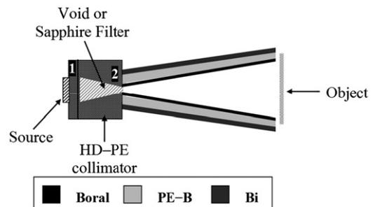
Fig. 2. The collimator geometry for thermal neutron radiography with the sapphire filter in front of the collimator (not in scale).
