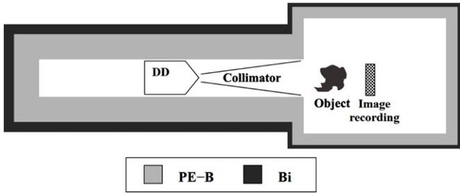
Fig. 1. Side view of the geometric configuration of the irradiating system (not in scale).
