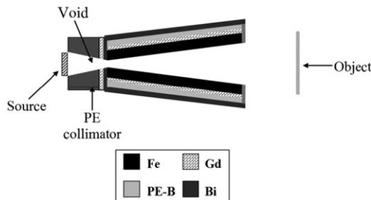
Fig. 3. The aperture geometry and the collimator for fast neutron radiography (not in scale).
