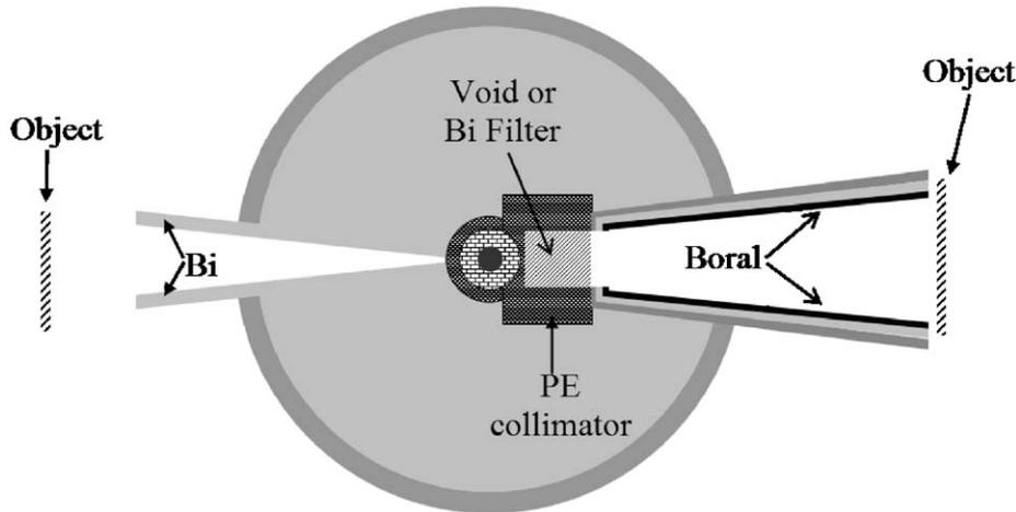
Fig. 2. Geometric configuration of the suggestion layout with the two different types of collimators—not in scale.
