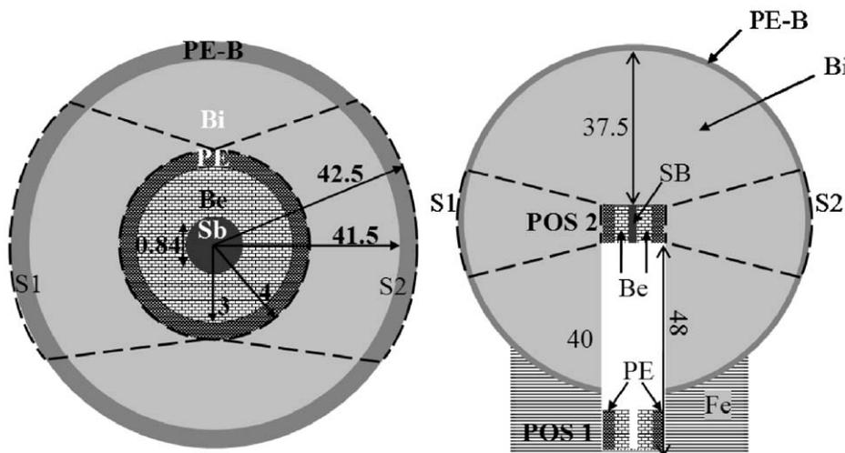
Fig. 1. Top and side view of the mobile SbBe source—not in scale (all dimensions in cm).
