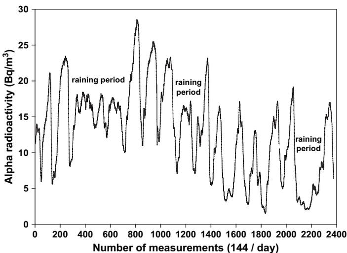
Fig. 4. Concentration of gross  $\alpha$ -air radioactivity over 15 days.
