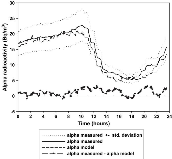
Fig. 5. Modelling of  $\alpha$ -radioactivity in air near the ground as a function of meteorological conditions and ground level  $\gamma$ -radioactivity.
