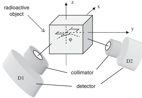
Fig. 1. The arrangement of two collimated detectors and a cubic radioactive object.
