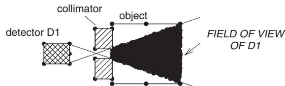
Fig. 2. A geometrical plot of the field of view of detector D1.
