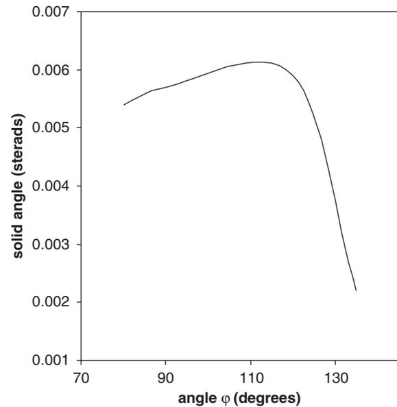
Fig. 4. Variation of the solid angle that detector D2 subtends at the area of intersection as a function of the rotation angle  $\varphi$ .
