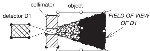
Fig. 5. The effect of self-absorption on the field of view of detector D1.
