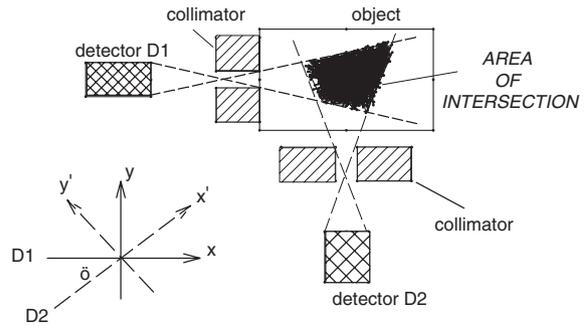
Fig. 3. A geometrical plot of the area of intersection between D1 and D2.
