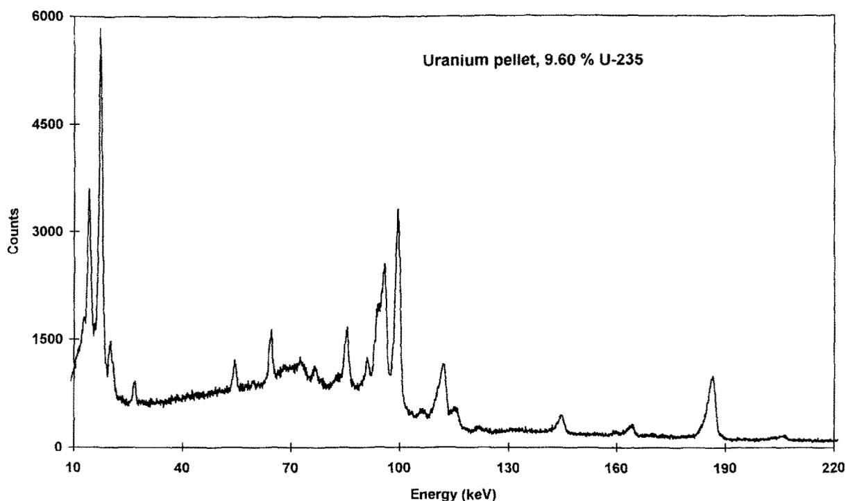
Fig. 4.  $\gamma$  spectrum of fuel pellet of uranium of 9.60% enrichment obtained with the CdZnTe detector.
