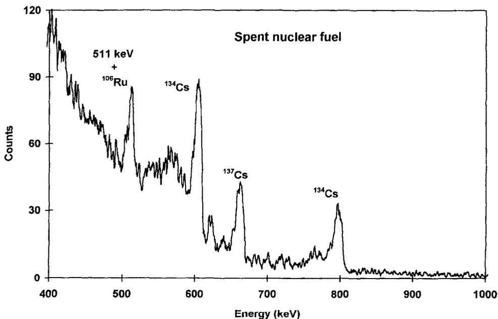
Fig. 1.  $\gamma$  spectrum of spent nuclear fuel obtained with the CdZnTe detector.
