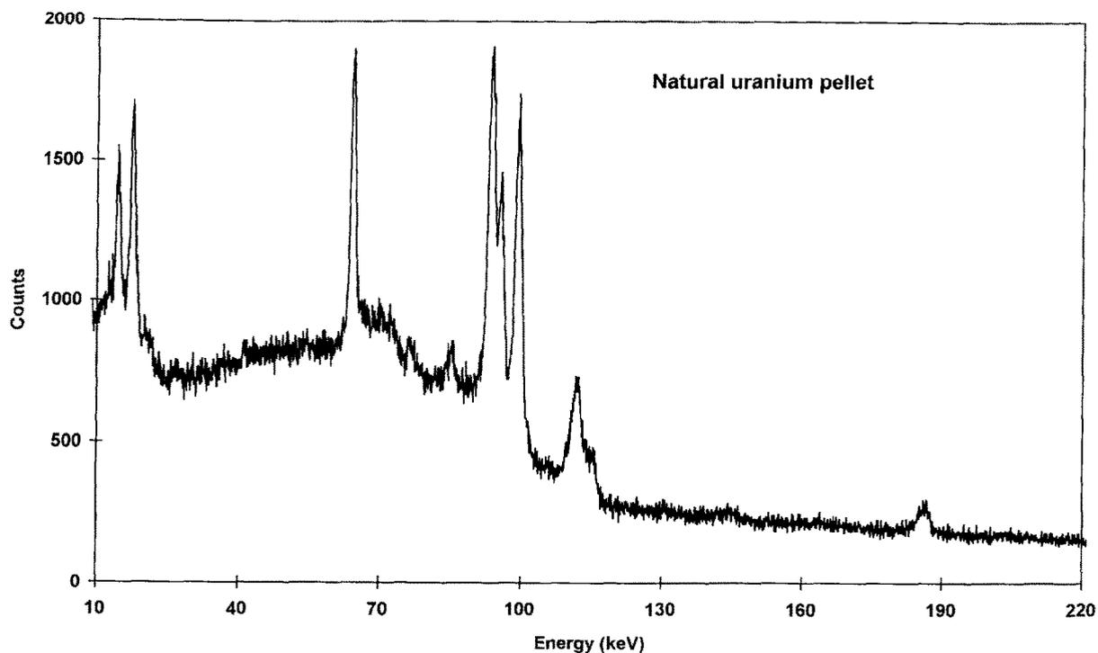
Fig. 3.  $\gamma$  spectrum of fuel pellet of natural uranium obtained with the CdZnTe detector.
