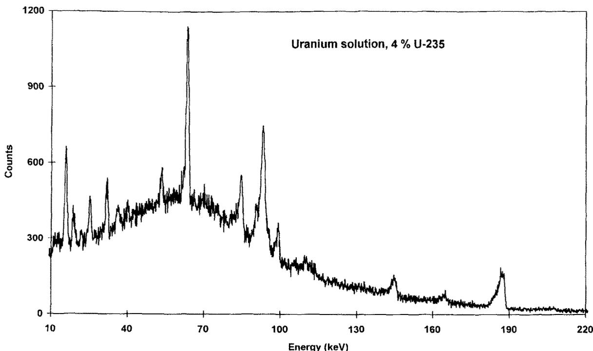
Fig. 2.  $\gamma$  spectrum of nitric acid solution of uranium of 4% enrichment obtained with the CdZnTe detector.
