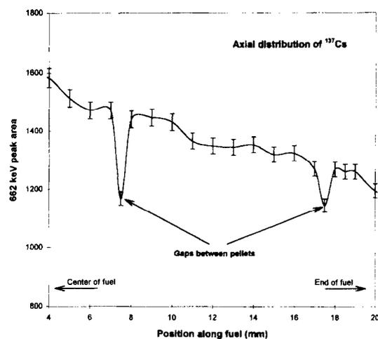
Fig. 4. Axial distribution of the  $^{137}\text{Cs}$  along the spent nuclear fuel rod showing the gaps between successive pellets.
