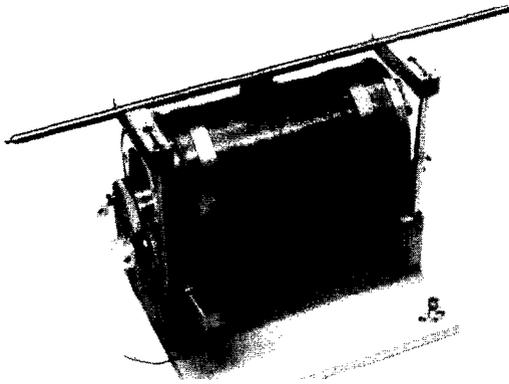
Fig. 1. Picture of the monitor with the collimator and dummy fuel rod in position.
