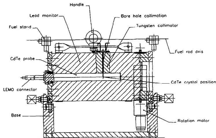
Fig. 2. A side view design of the monitor where the most important components are indicated.
