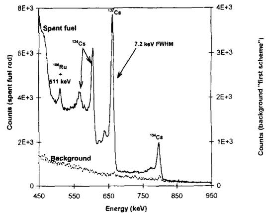
Fig. 3. Gamma spectrum of a spent nuclear fuel rod and the background obtained inside the hot cell.
